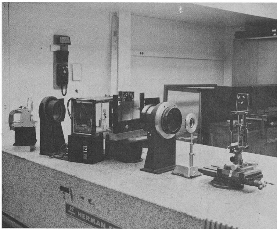
FIG. 3. The experimental system. The test section, hologram, and viewing system can be seen in the foreground.
